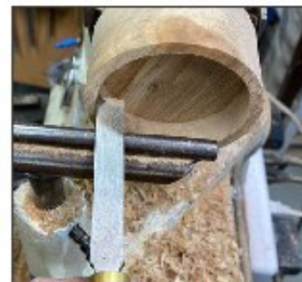
Cut the box's walls parallel with a flat-end scraper so that the lid will fit properly.
