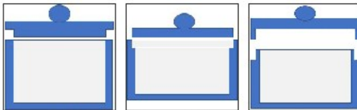
Figures 1, 2, 3. Loose lids generally have a short tenon that fits into the opening of the box, either protruding above the sides of the box (Type 1, left ), or flush with the box sides (Type 2, center ). Although Type 1 and Type 2 boxes can be made with tight lids, it is more common to see Type 3 ( right ) boxes with a lid that fits snugly so that it can be carried around without falling open.
